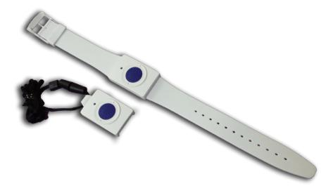
Our standard **Emergency Transmitters** can be worn as a pendant or on the wrist like a watch. They are waterproof, and can be worn at all times, even when in the shower.
